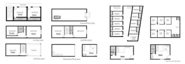
Fig. 7 - Typical layouts of a mini – appartments for workers to rent (Source: Pham, D.T., 2015)
