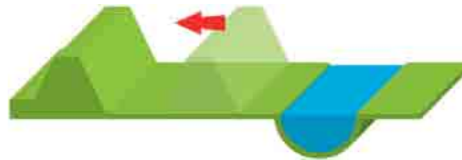
Main measure in Room for the River Waal: Dyke relocation
